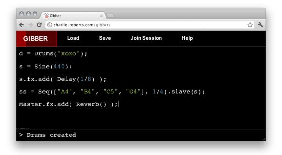
**Figure 1**. Gibber running inside of Google Chrome. The red bar in the upper left is a metronome indicating the current beat in 4/4 time; beat one is currently highlighted.
